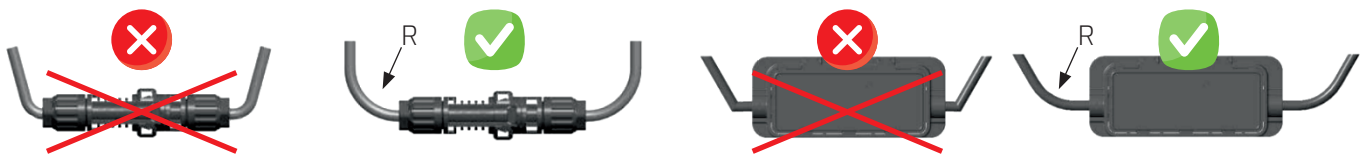
Fig. 5: permissible bending radius of the solar cables
